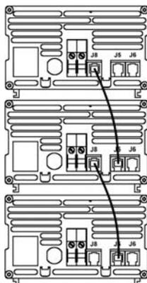
Bus cables can be connected from previous units to the next with the same way. The first unit must be the master unit (with adjusting knobs). Wrong connection does not damage the units but in that case slaves does not follow the master's commands. Quantities of the slave units are unlimited.
