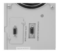
Use the 9 Pin communication cable to connect the UPS and equipment to implement the remote monitor and control.
