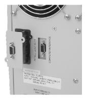
The cover of AS400 card should attach close to the rear panel. Then fixing it by using screws.
