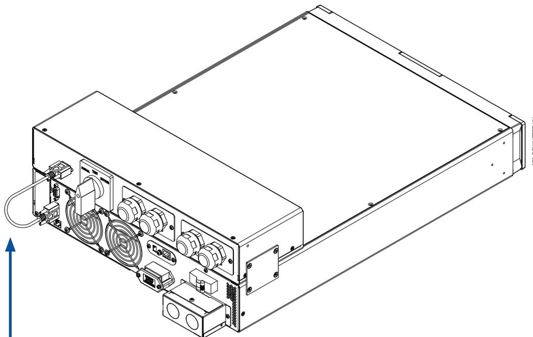
Ensure parallel cable with DB9 connectors is installed between bypass switch and UPS.
