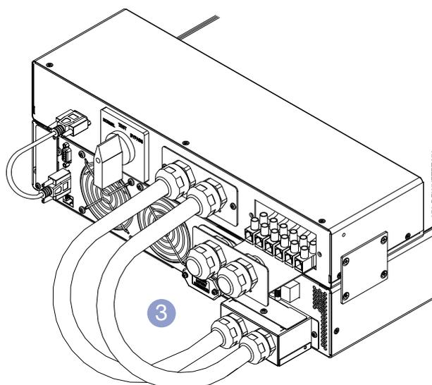
6.2.5 Connection of cables to the BY-PASS input and output terminal strips
