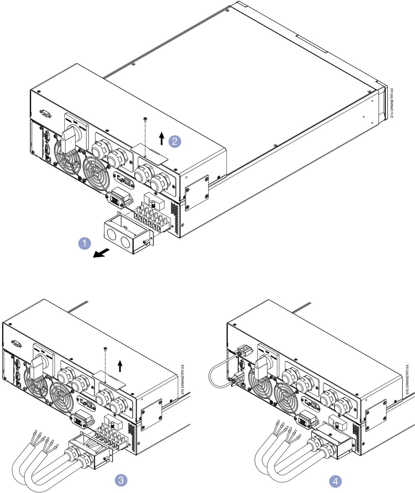
6.2.4 Connection of cables to the BY-PASS terminal strips
