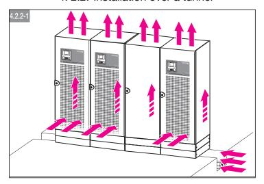
4. 2.3. Heat loss and ventilation characteristics
