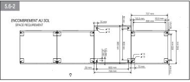
Each foot has a floor fixing hole (labelled A : Ø 13) and welded nut for level adjusting (labelled B : screw THM 12 not supplied).
