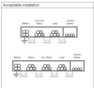
1. Control cables: connections between the cabinets and each unit, alarm signals, remote mimic panel, connection to the BMS (Building Management System), emergency stop, connection to generator.
